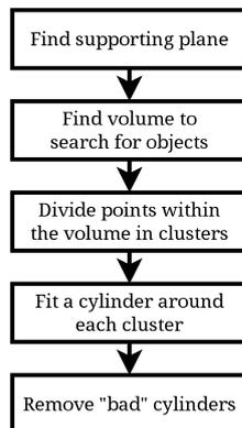
Figure 4: The main steps in the object detector.
