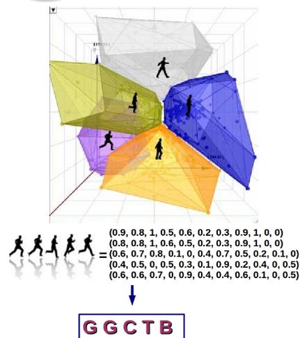
Figure 2: Example of posture quantization using clustering, where each posture of the series was initially a vector of 11 real values. After clustering, we obtain a single tag.
