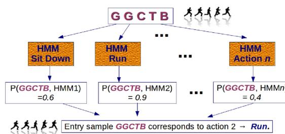
Figure 3: Example of action recognition with the trained HMMs.
