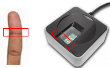
Figure 3: Guide on the proper placement of a finger on the FS88 scanner: align the lines inside the red rectangles.
