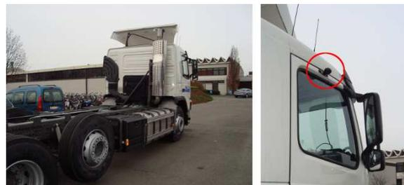
Figure 11: Our test truck with the mounted commercial blind spot camera (circled in red).
