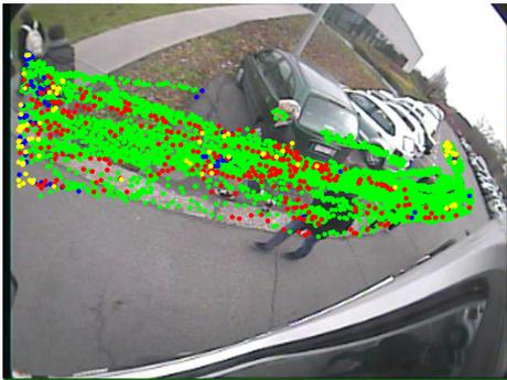
Figure 8: Performance of the two transformation models in function of the position. Colored dots indicate which model performed the detection. Red: perspective model. Blue: similarity model. Green: both models. Yellow indicates missed detections.
