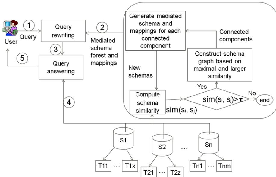
Figure 2: A query system with hierarchical mediated schemas.
