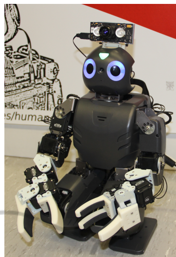
Figure 5: The DarwinOP robot has been modified with grippers and a depth camera. The control system has been completely rewritten to take advantage of the embedded PC/micro-controller architecture.
