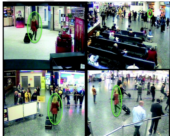
Figure 1: Person re-identification task: the system should be able to match appearances of a person of interest extracted from non-overlapping cameras.
