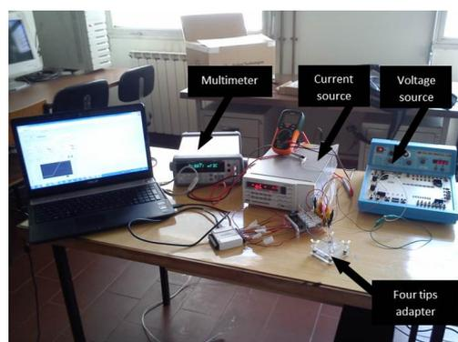
Figure 10: Experimental setup for the resistivity measurements (including a multimeter, current and voltage sources and a four tips adapter).
