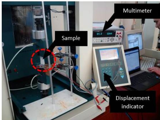
Figure 12: Experimental setup for the mechanical tests.
