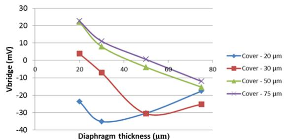
Figure 6: Voltage output of the Wheatstone bridge according to the thickness of the diaphragm and the PDMS cover layer, for Aluminium strain gauges (200 nm thickness) and a pressure signal of 225 mmHg.
