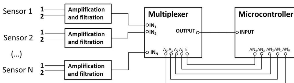
Figure 9: Different blocks that constitute the readout system and their connections. The sensors can be seen in Figure 4.
