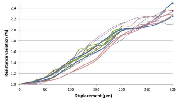
Figure 13: Displacement versus resistance change for gold films deposited in PDMS.
