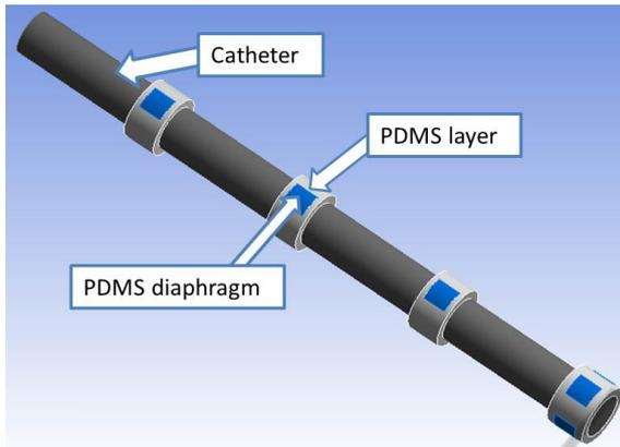
Figure 1: Catheter and the respective PDMS layers along it (diaphragms are highlighted). At the tip, four diaphragms are machined for intrasphincteric measurements.
