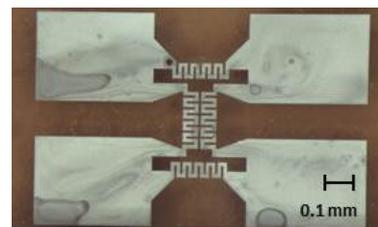
Figure 8: Aluminium strain gauges embedded in PDMS.
