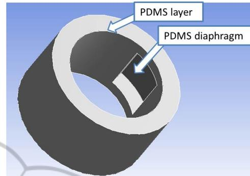
Figure 2: Representative section of the catheter with a diaphragm machined in the structure (centre of the structure).
