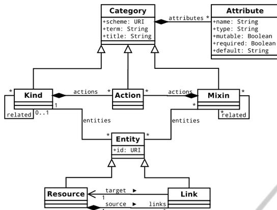
Figure 1: The OCCI core model – A UML class diagram
