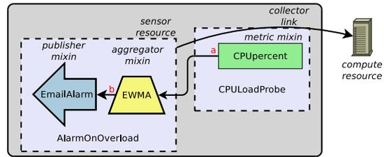
Figure 3: Block representation of a CPU overload alarm.
