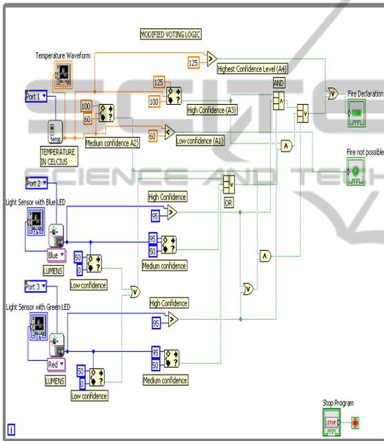
Figure 8: LabVIEW implementation of Modified Voting Logic.
