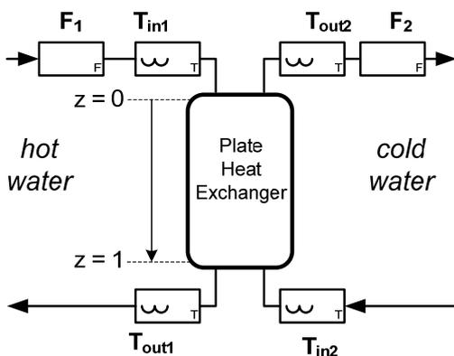
Figure 1: Schematic diagram of the considered PHE setup.
