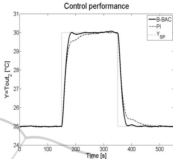
Figure 3: Tracking properties of the considered controllers. Noisy case.
