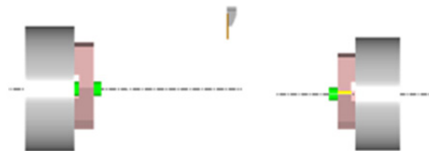
Figure 21: Work piece is moved from main spindle to sub-spindle.
