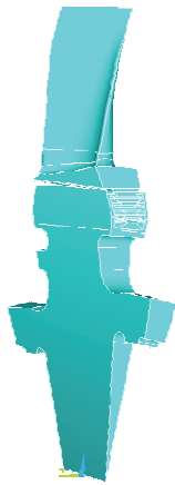
Figure 5: Computational model for turbocharger TK-32 turbine rotor wheel's strength analysis.
