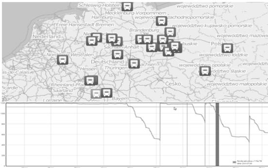
Figure 3.2: Screenshots from the Fleet Management System. The top image presents the current position of the vehicles on the OpenStreetMap. The bottom image presents the plot of the fuel level in one vehicle for the selected period of the time.
