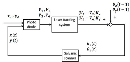
Figure 7: Block diagram of laser tracking system.
