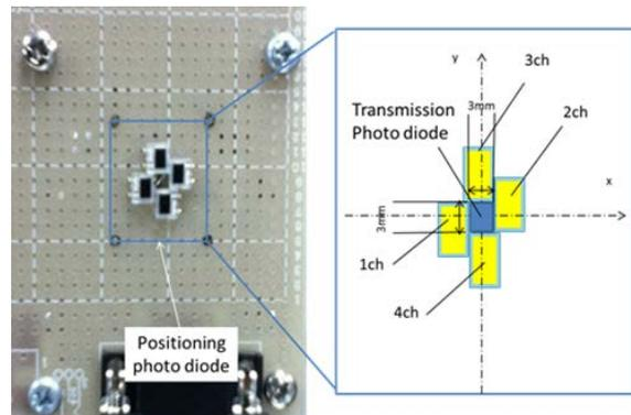
Figure 3: Positioning photodiode.
