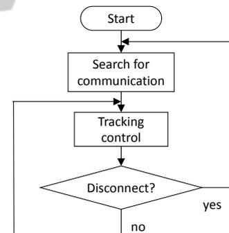
Figure 5: Laser beam alignment procedure.
