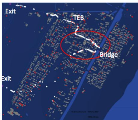
Figure 4: The last snapshot of simulation showing in white the areas of traffic congestion during evacuation. Traffic congestion was confirmed with survivors for the segment in front of the Tsunami Evacuation Building (TEB).
