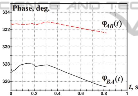
Figure 1: Examples of Phase-Time Responses of the same meteor radio reflection observed at both sides of the link
