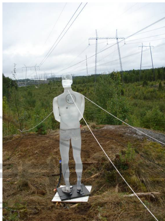
Figure 1: The phantom under the power line (in place B).
