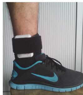
Figure 6: IMU Device mounted close to the ankle.
