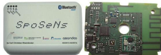
Figure 3: Sensor unit (left) and board (right).
