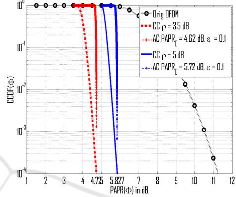
Figure 12: Comparison of CC and AC in terms of PAPR reduction for different thresholds  $\rho = 3.5\text{dB}$  and  $\rho = 5\text{dB}$ .
