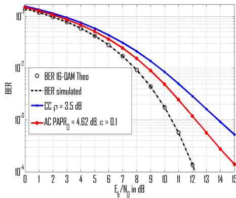
Figure 13: Comparison of CC and AC in terms of BER degradation for  $\rho = 3.5$  dB.
