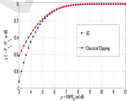
Figure 9: Comparison of CC and AC in terms of mean power degradation
