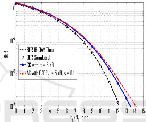
Figure 8: Comparison of CC and AC in terms of BER degradation for  $\rho = 5\text{ dB}$ .
