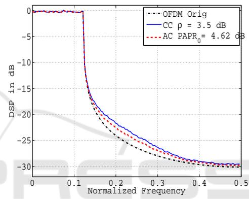
Figure 16: Comparison of DSP of the AC and CC methods for  $\rho = 3.5$  dB.
