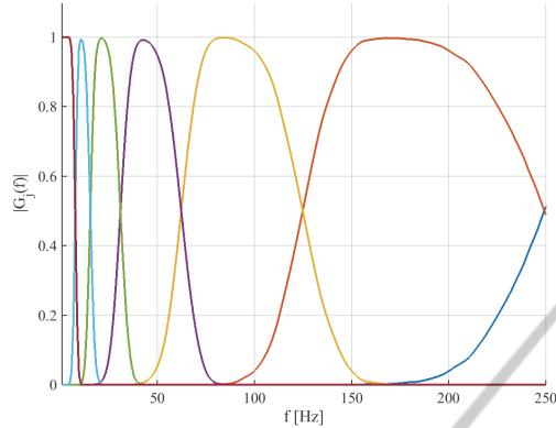
Figure 2: Frequency response of different scales of the dyadic discrete Wavelet Transform.
