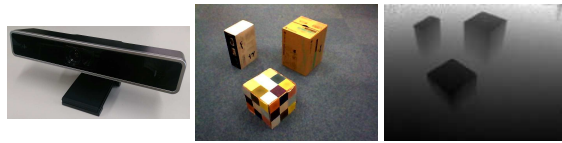
Figure 1: Left: SoftKinetic DepthSense DS311. Center: captured color image. Right: captured depth image.
