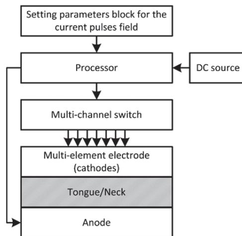
Figure 1: Block diagram of the engineering feasibility of multi-channel neurostimulation systems.
