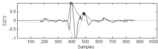
Figure 3: Example of the temporal positive and negative contour envelopes of a S2.
