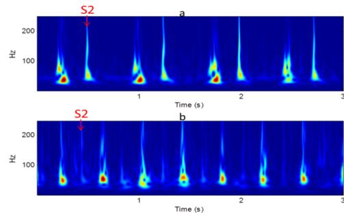
Figure 4: The S-Transform of two sounds corresponding to the same subject and two different heart rates (a: HR=80 bpm, b: 142 bpm) showing the high frequency content of S2 decreases when the heart rate is higher.
