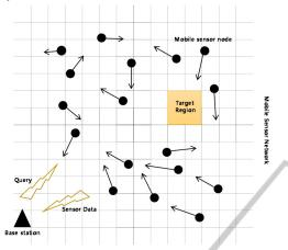
Figure 1: Mobile sensor network with randomly moving sensor nodes.
