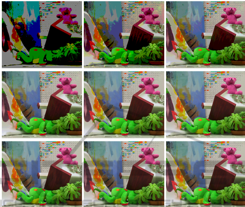
Figure 2: 24-bit RGB color image bit-plane sliced into 8 layers. From top-left to bottom-right: layer 1, layer 2, ..., layer 8, and the original image.
