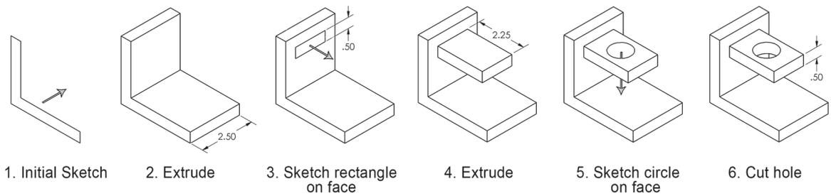
Figure 4. Modeling steps to create sample part.
