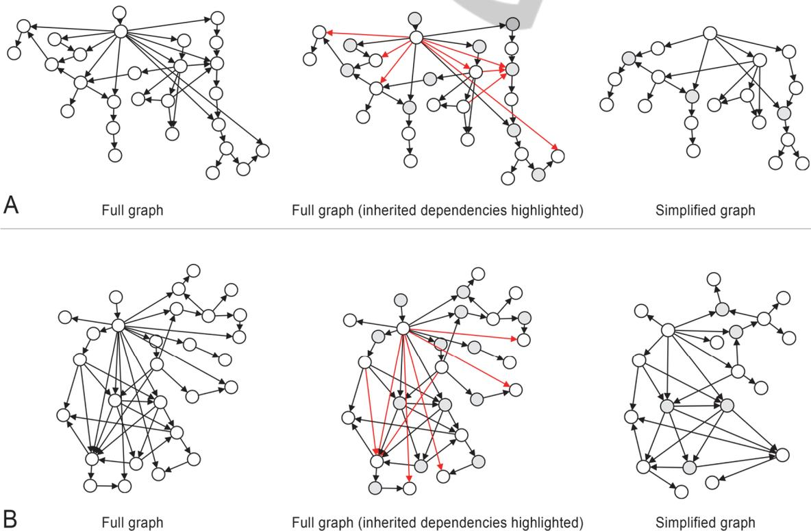
Figure 9: Comparison of the full graph and simplified version for two CAD models (A and B). Node names have been omitted for clarity.
