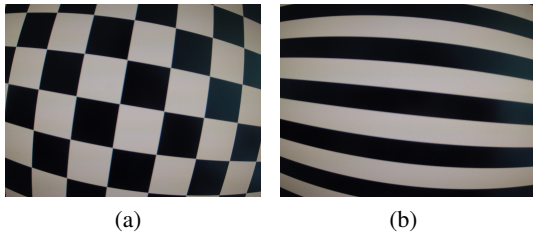
Figure 1: Periodic calibration patterns, the checkerboard (a) and the parallel line bundle (b).
