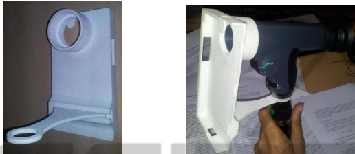
Figure 5: (a) RP model of Case and (b) Ophthalmoscope attached with mobile phone holder.
