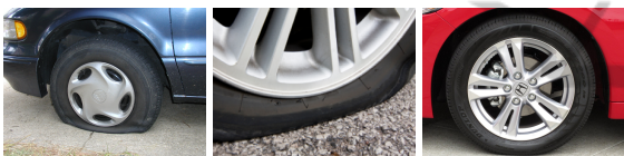
(a) Tire is flat. (b) Tire is under-inflated. (c) Tire is OK. Figure 3: The perception system must be able to determine whether a tire is really flat, and which one it is.
