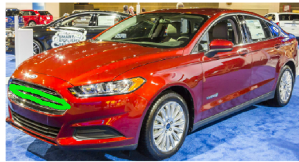
Figure 10: With insufficient guidance, the Hough algorithm finds an ellipse in the car's grill (highlighted in green), rather than finding the wheel.
