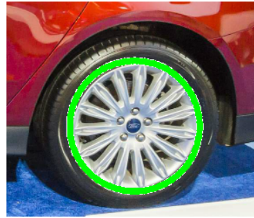
Figure 15: Successful Hough ellipse match to rear wheel (match highlighted in green).
