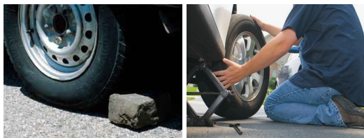
(a) Wheel chock. (b) Remove wheel. Figure 4: Repair steps include stabilizing the car (a), getting the spare tire and tools, jacking up the car, removing lug nuts and wheel (b), and installing the new wheel.
