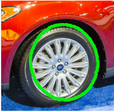
Figure 18: Successful Hough ellipse match, using ellipse rather than circle variation of the algorithm.
