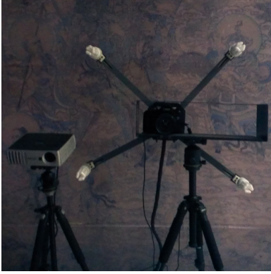
Figure 1: Our setup. Our experimental setup consists of a digital camera, four lights and a digital light projector. We use the camera for both photometric stereo and structured-light scan.
