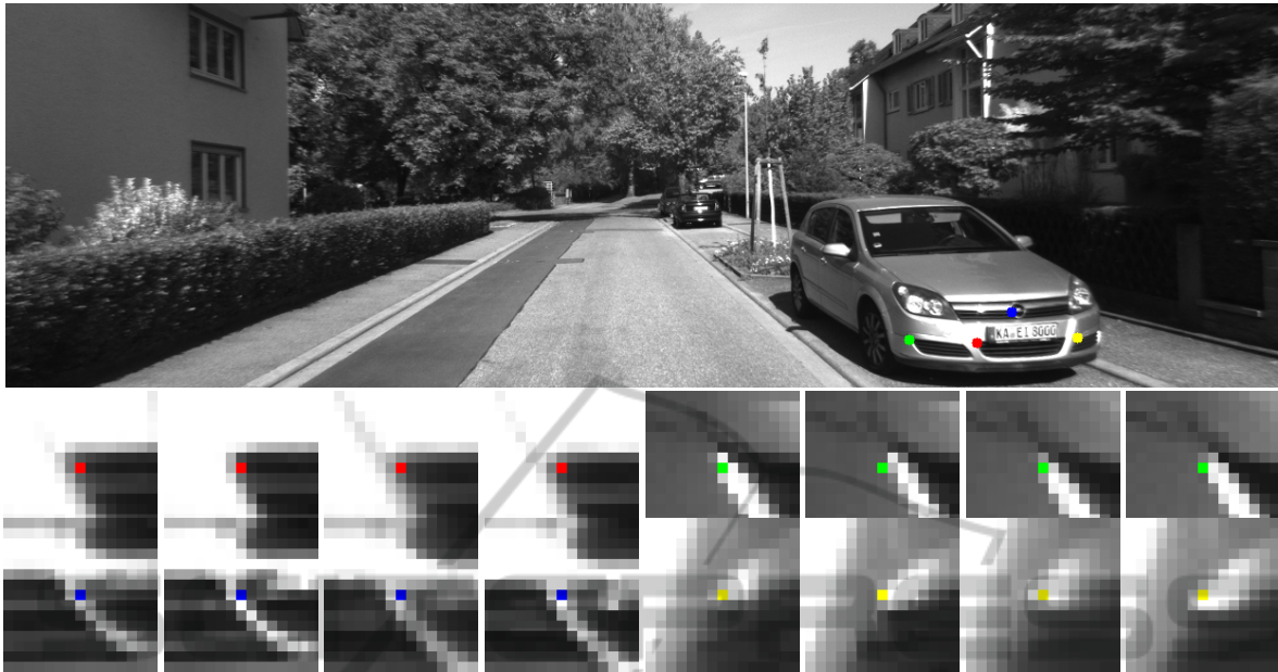
Figure 2: The image on the top corresponds to the frame #1 of the training KITTI sequence 03. Four point features have been annotated with different colors. The four bottom images show four 15x15 patches around each feature point in four different images (current-left, current-right, previous-left, previous-right). The localization error in the four images is less than 1 pixel. However, the reprojection errors evaluated for groundtruth motion are around 7 pixels as shown in Table 1.
