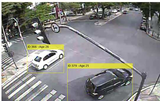
Figure 6: Vehicle ID and age computed by tracking methodology.
