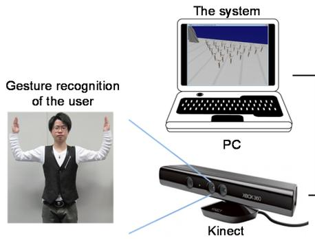
Figure 1: Configuration of system.
