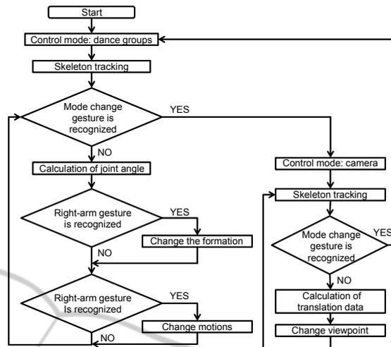
Figure 2: Process of gesture recognition.
