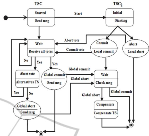
Figure 8: State diagram of the proposed protocol.
