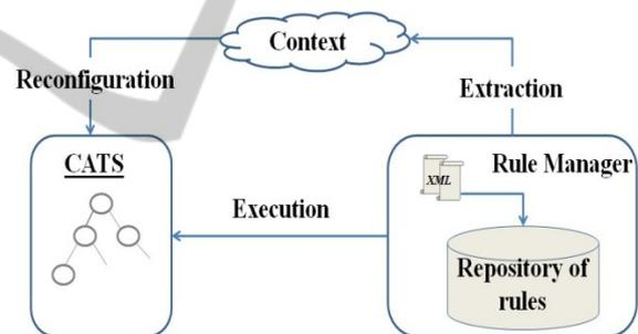
Figure 2: Adaptation approach by rules specification.
