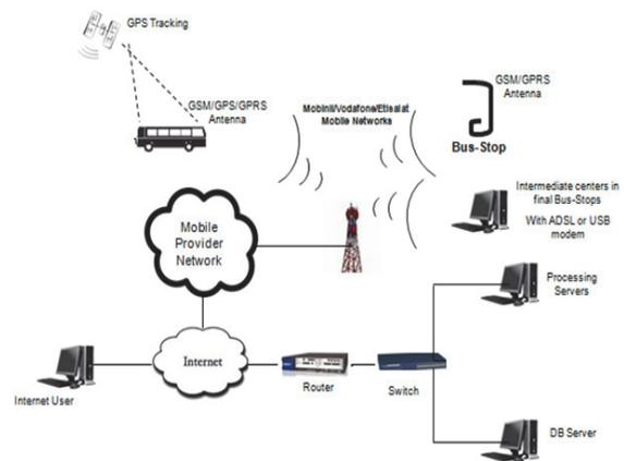
Figure 1: Main structure of proposed system.
