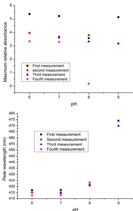
Figure 13: The maximum value of the relative absorbance (up) and the peak wavelength (down) versus pH for the consecutive measurements of the pH solutions for (PAH/BY)<sub>6</sub>APTMS on the glass slide. The sample was cured at 120°C for 4 hours (The sample designated GS10).
