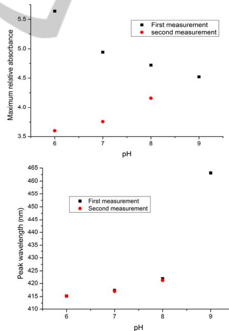
Figure 12: The maximum value of the relative absorbance (up) and the peak wavelength (down) versus pH for the consecutive measurements of the pH solutions for (PAH/BY)<sub>6</sub>(APTMS/SiO<sub>2</sub>)<sub>2</sub> on the glass slide. The sample was cured at 120°C for 4 hours and examined after a week (The sample designated GS09).
