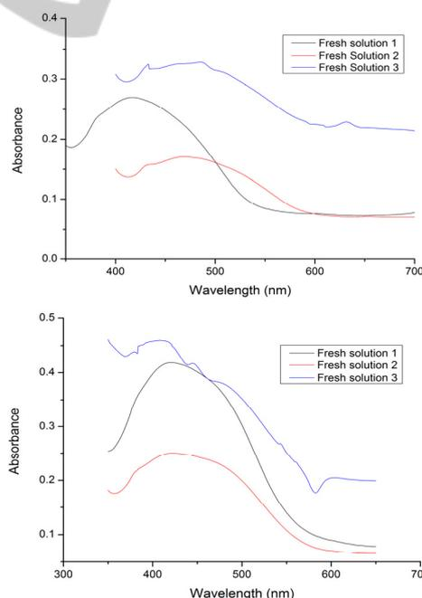
Figure 14: The spectra for the coated glass slides with (PAH/BY)<sub>6</sub> dipped into the fresh buffer solution for three times and each time for 60 minutes. Up: pH 6 (The sample designated GS11), Down: pH 8 (The sample is designated GS12). The samples were cured at 120°C for 4 hours.
