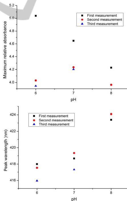
Figure 2: The maximum value of the relative absorbance (up) and the peak wavelength (down) versus pH for the consecutive measurements of the pH solutions for (PAH/BY)<sub>8</sub> on the glass slide. No heat treatment or drying was used in the process (The sample is designated GS01).
