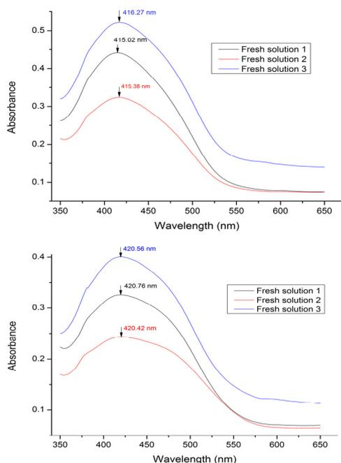
Figure 15: The spectra for the coated glass slides with (PAH/BY)<sub>6</sub>(APTMS/SiO<sub>2</sub>)<sub>2</sub> dipped into the fresh buffer solution for three times and each time for 60 minutes. Up: pH 6 (The sample is designated GS13), Down: pH 8 (The sample is designated GS14). The samples were cured at 120°C for 4 hours.
