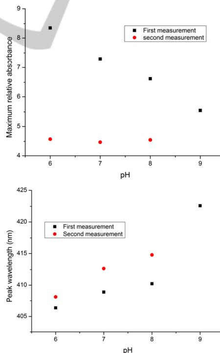
Figure 8: The maximum value of the relative absorbance (up) and the peak wavelength (down) versus pH for the consecutive measurements of the pH solutions for (PAH/(BY+SiO<sub>2</sub>))<sub>6</sub> on the glass slide. The sample was cured at 120°C for 4 hours (sample designated GS07).
