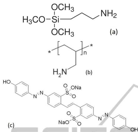
Figure 1: Chemical structure of (a) APTMS, (b) Poly(allylamine) hydrochloride [PAH] and (c) brilliant yellow.
