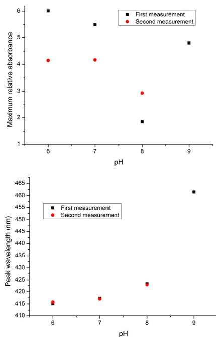
Figure 11: The maximum value of the relative absorbance (up) and the peak wavelength (down) versus pH for the consecutive measurements of the pH solutions for the (PAH/BY)<sub>6</sub>(APTMS/SiO<sub>2</sub>)<sub>2</sub> on the glass slide. The sample was cured at 120°C for 4 hours (The sample designated GS08).
