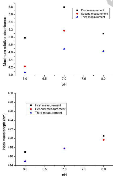
Figure 3: The maximum value of the relative absorbance (up) and the peak wavelength (down) versus pH for the consecutive measurements of the pH solutions for (PAH/BY)<sub>16</sub> on the glass slide. The sample was cured at 120°C for 4 hours (The sample is designated GS02).
