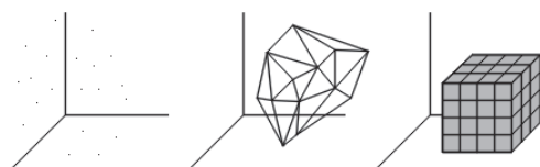
Figure 1: Point-based, surface-based and solid-based models (point cloud, wireframe and voxels).
