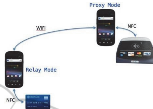
Figure 7a: Diagram of a Remote Relay attack (source: Lee, 2012).
