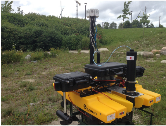
Figure 6: Overview of the Kingfisher Robotics Platform. The unmodified platform comes equipped with an IMU, a GPS antenna, a radio transceiver and differential drive capability. Additional sensing capabilities have been added to the platform, these include a panoramic array of camera and a SONAR depth sensor.
