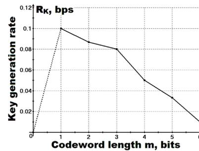
Figure 5: Key generation rate as a function of the codeword length.
