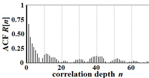
Figure 4: Autocorrelation function of the collected sample of carrier phase measurements.
