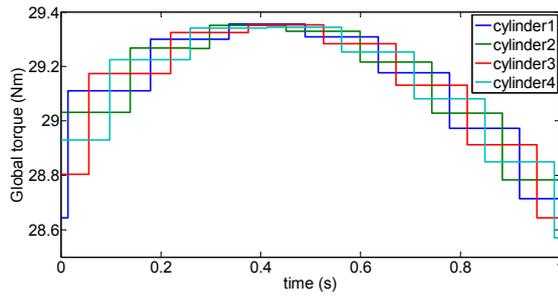
Figure 7: Individual cylinder torque observer results.
