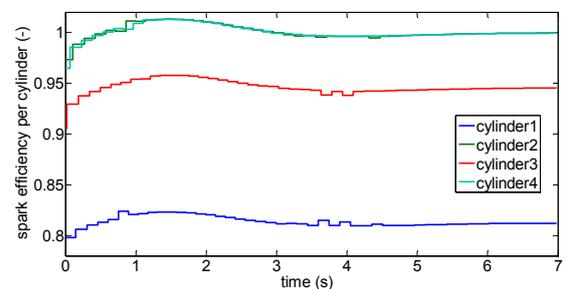
Figure 11: Individual spark advance efficiency observer results with two imbalances.
