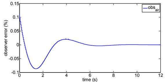
Figure 6: Air mass observer error in percentage.
