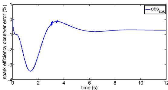
Figure 9: Individual spark efficiency observer error.
