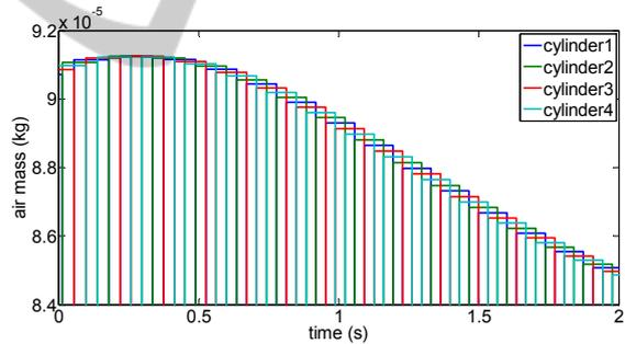
Figure 5: Individual cylinder air mass observer results.
