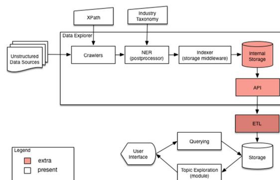
Figure 3: High-level Architecture of the prototype.
