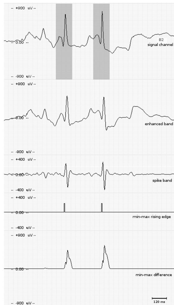
Figure 1: Illustration of first level detection method: B2 is a regular signal channel with two detected spikes; 'enhanced band' is filtered by bandpass 1-35 Hz; 'spike band' is filtered by bandpass 20-50 Hz; min-max rising edge illustrates threshold crossing points.
