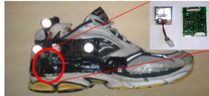
Figure 1: Shoe with IMU and Jig for facilitating ground truth capture using the Vicon Motion capture system.
