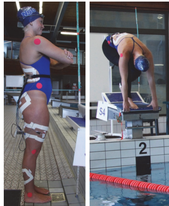
Figure 3: Swimmer with fixated electrodes and markers and the MQ16 on the back. OSB11 cover with pressure mat placed under the front foot.
