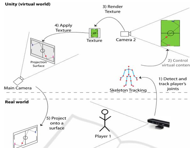
**Fig. 8.** Human interactions. One or two humans are tracked simultaneously using Kinect's skeleton tracking (step 1). The corresponding joint, for each player, controls the respective virtual object (step 2). Camera 2 renders the texture containing the view of the camera (step 3) that is then applied to one of the projection surfaces and updated in runtime (step 4). The final step can now take place: project onto one real world surface (step 5).
