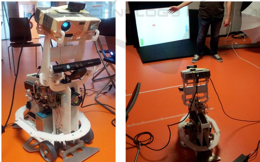
**Fig. 9.** Augmented reality on Wheels – Content is projected onto multiple surfaces in order to help user perform actions, or to play games with users (such as the Air Hockey game, as shown in the right image).
