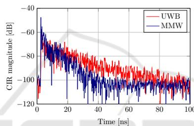
**Fig. 14.** Comparison of mmW CIR with UWB CIR [23].
