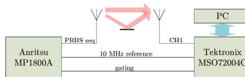
**Fig. 11.** PRBS based measurement setup [20].
