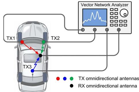
**Fig. 6.** UWB MISO measurement setup [17].
