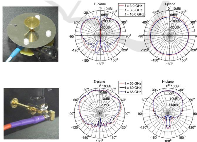
**Fig. 2.** Antenna used for UWB (top) and mmW (bottom) measurements with corresponding radiation patterns.
