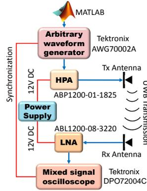
Fig. 3. UWB time domain measurement setup [14].
