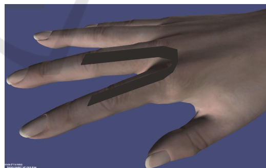
Figure 1: Strip rectangular flex sensor upright the dorsal aspect of two adjacent fingers to measure abduction/adduction angles.
