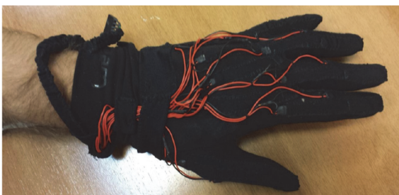
Figure 2: Lycra-based glove. Signals from only three flex sensor were used in this work.
