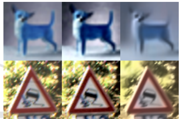
Figure 2: Examples of images from CIFAR-10 and GTSRB in order: original, pixel intensity equalization, non-local means denoising.
